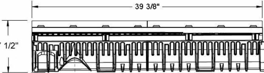
100C HD Presloped Channel with DI Frame ( Preslope Upgrade )
